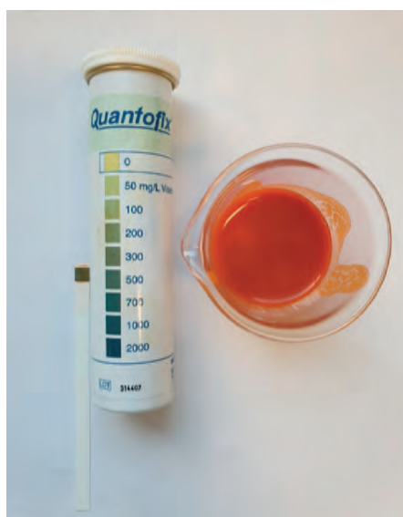
Vitamin C test strip and scale after immersion in goji berry juice
