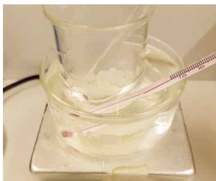
Oily phase ingredients are placed in a beaker inside a water bath and mixed using a magnetic stirrer or glass rod.
