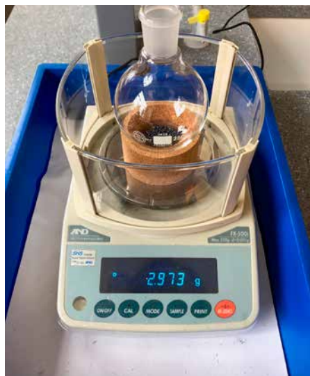
Weighing the iodine (step 1)
