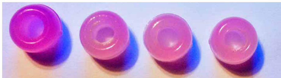
Colour intensities of UV beads exposed to UV light, from left to right: without sunscreen; with SPF 20; SPF 50; SPF 90.
