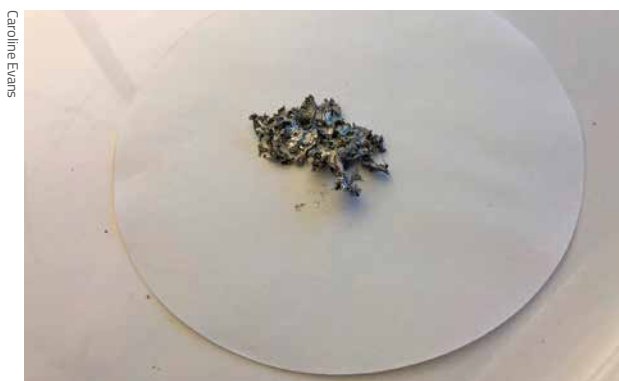
Leftover tin, dried on filter paper (step 13)
