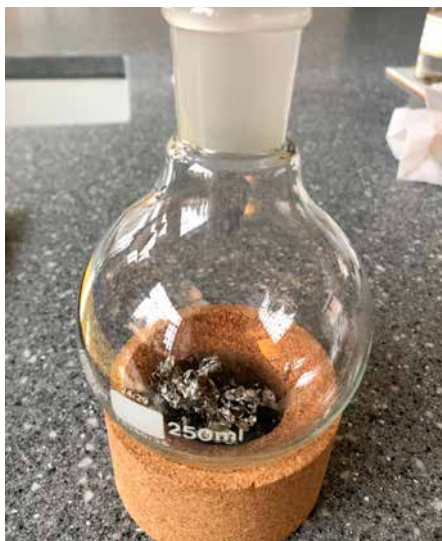
Tin and iodine in the flask (step 2)
