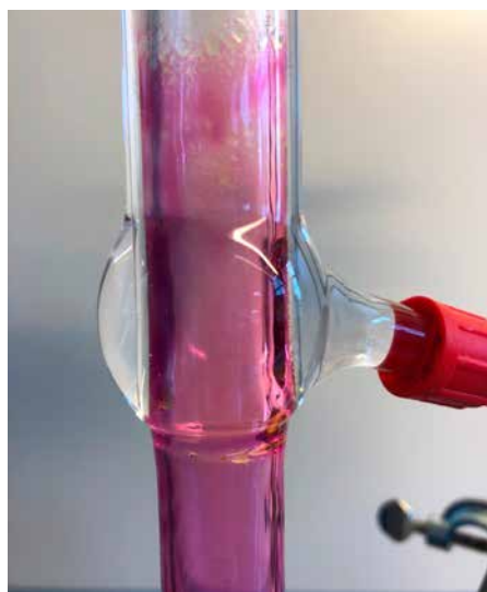
Iodine vapour in the reflux condenser
