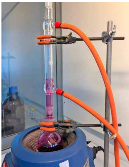
Iodine vapour rising as the mixture is heated (step 7)
