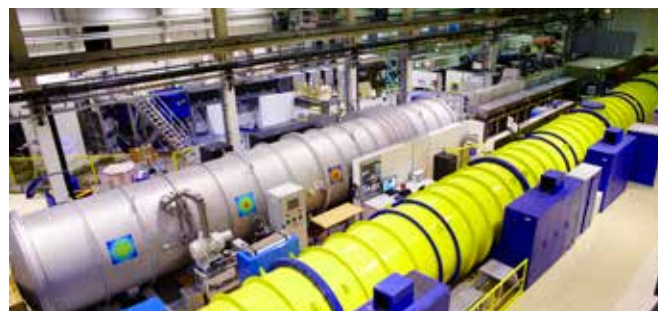
The D11 neutron scattering instrument, which was used to study the molecular structure of limoncello
