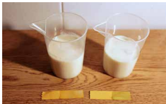
Figure 2: pH indicator strips show a decrease from 7 (neutral) to 6 (slightly acidic) between the test on the right (without enzymes, the green indicator strip) and the lipase-containing test on the left (the yellow indicator strip).
