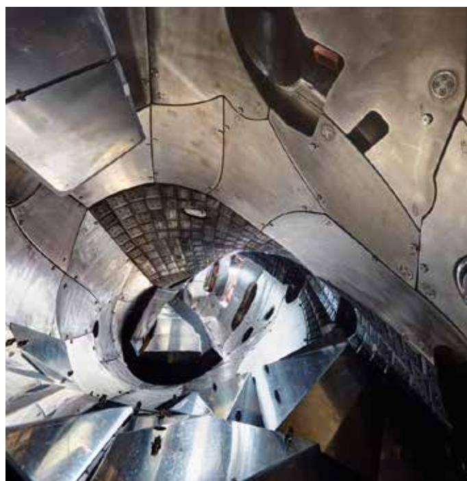
A view inside the plasma vessel of the Wendelstein 7-X fusion device
