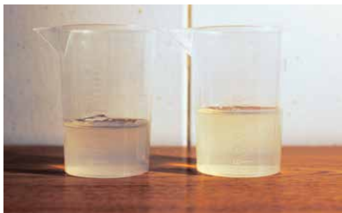
Figure 1: The solution on the left contains protease, which results in a visible decrease in the level of the gel in comparison to the test on the right, which contains no enzymes.
