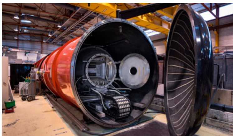
The D22 instrument at ILL, which revealed how water and ectoine interact with protein surfaces. The door of the apparatus has been opened to show a view of the neutron detector.
