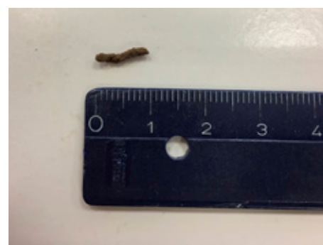
Figure 8: Grinding three pieces of dried rubber produces an eraser roughly 1 cm in length.
