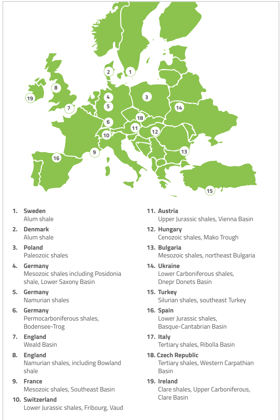
Figure 2: Map showing location of potential shale gas reserves across Europe. (Source: Hans-Martin Schulz, GFZ Potsdam)
