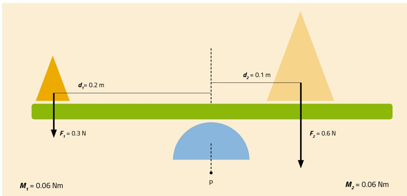
Figure 3: For a tray to remain balanced, the total anticlockwise moments ( $M_1 = F_1 \times d_1$ ) should be equal to the total clockwise moments ( $M_2 = F_2 \times d_2$ ) so  $F_1 \times d_1 = F_2 \times d_2$ . P: pivot
