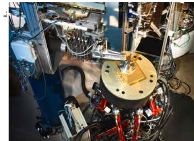
ILL's SALS instrument performs diffraction experiments with engineering applications
