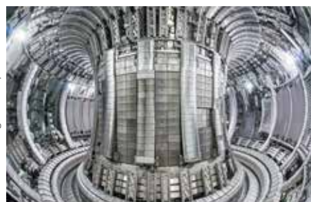
An internal view of the reaction vessel of the Joint European Torus (JET)
