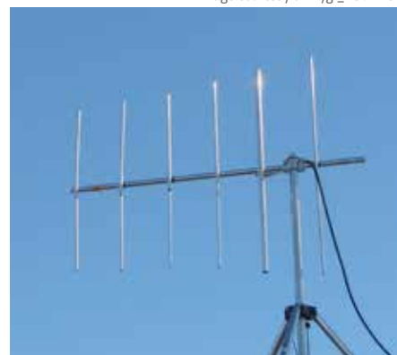
Figure 1: Yagi radio antenna
