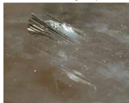
Figure 2: The reverse side of the same sample. Although not visible from the side that was impacted, the damage is catastrophic.
