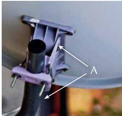
Figure 1: Remove the mount (A) at the back of the satellite dish
