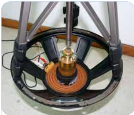
Figure 6: Our homemade geophone
