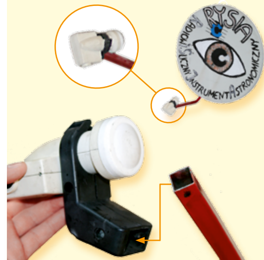
Figure 4: Attaching the LNB to the antenna arm
