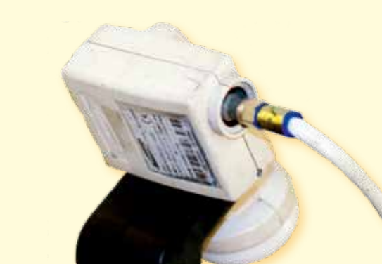
Figure 8: Powering the satellite meter and receiving the signal from the LNB
