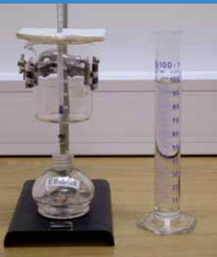
Alcohol burner set up under a beaker to which a known volume of water is to be added
