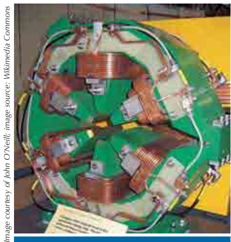
Sextupole magnets are used for correcting the beam size and position
