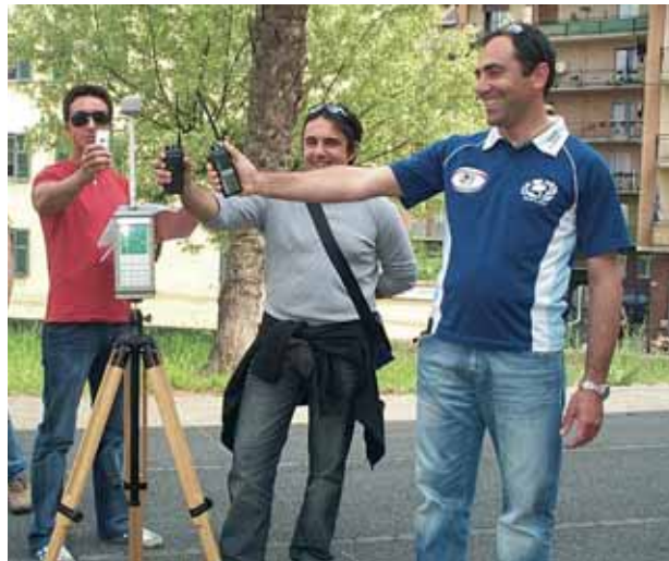
Students at the IIS “Deambrosis-Natta” testing electromagnetic hazards associated with hand-held radio devices
