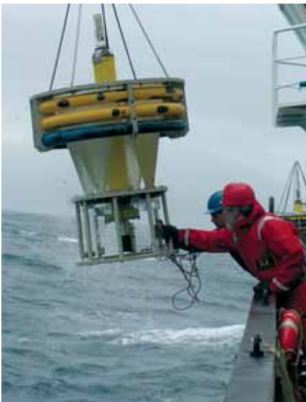
Measuring marine snow: RRS Discovery deploying a sediment trap west of the English Channel to capture sinking marine snow and analyse its composition
