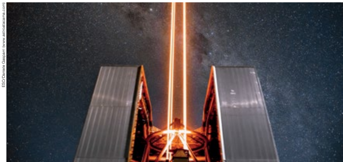
The adaptive optics system of Yepun (Unit Telescope 4 of the VLT) in operation.
