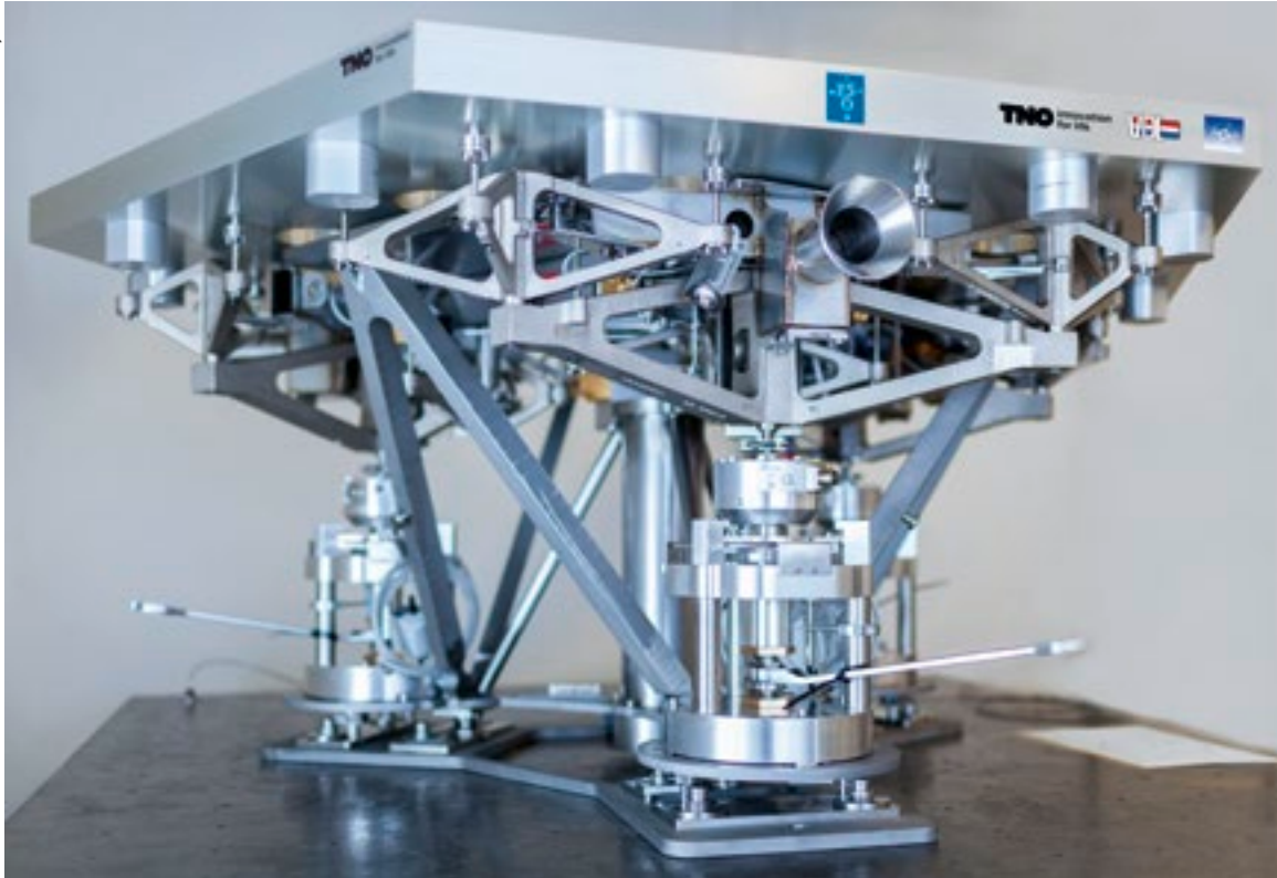
Figure 2. One segment support structure of the giant primary mirror of the ELT undergoing testing.
