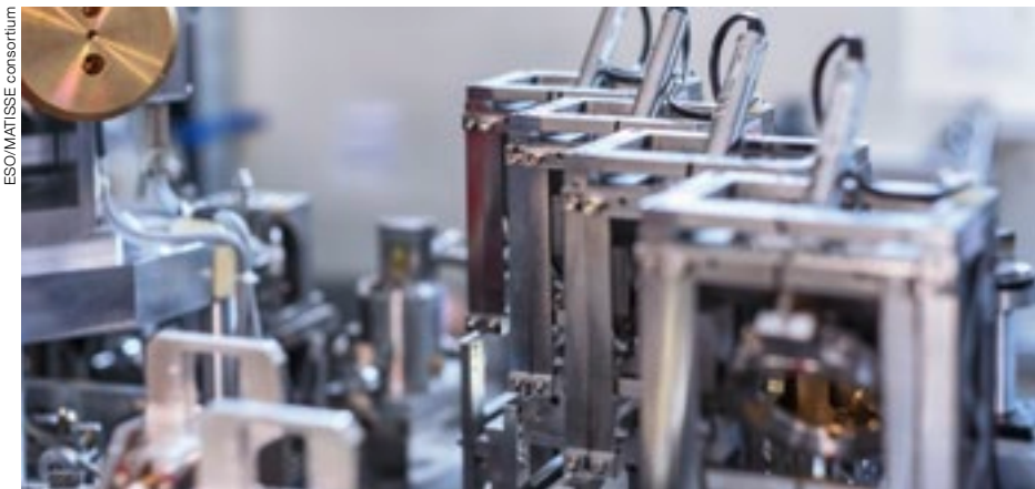
Complex optics on the MATISSE instrument on the VLTI. Many components are repeated four times, one for each beam of light being fed into the instrument.
