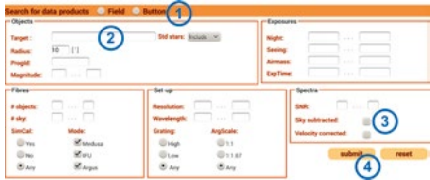
Figure 1. The GIRAFFE archive search interface is shown. The mandatory criterion Field/Button (1) must be specified. The other criteria are organised in five panels related to object information, exposure parameters, fibre configurations, instrumental set-up and spectral characteristics. See text for details.
