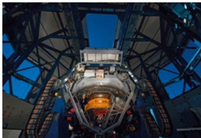
Figure 1. Left: The VST on the VLT platform. Right: OmegaCAM (the yellow volume) mounted on the VST.
