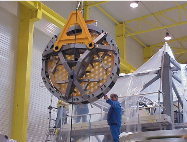
▲ Figure 3: The 1.8-m primary mirror in its cell during integration into the telescope at AMOS. The mirror is lightweighted to reduce its mass by a factor about 2. A 54-points waffle-tree axial support was selected to comply with the stringent image quality requirements.
