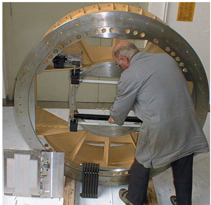
Figure 3: The 1.5-m diameter housing structure during a test assembly of the main units: the two storage magazines (to be inserted into the big shaft at left and hidden right), the filter exchange unit with the exchange carriage and a 420 × 320 mm 2 opaque, aluminium 'filter' (at the bottom left).
