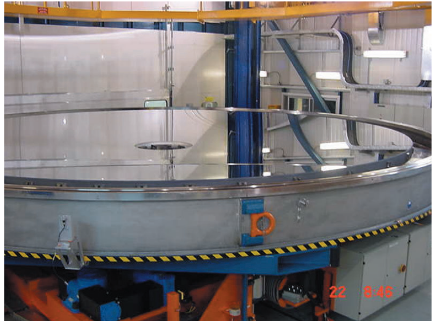
Figure 2: The primary of UT3 coming out of the coating chamber with a reflectivity of 92% and a micro-roughness of 7 Ångströms. The best coating ever at Paranal.
