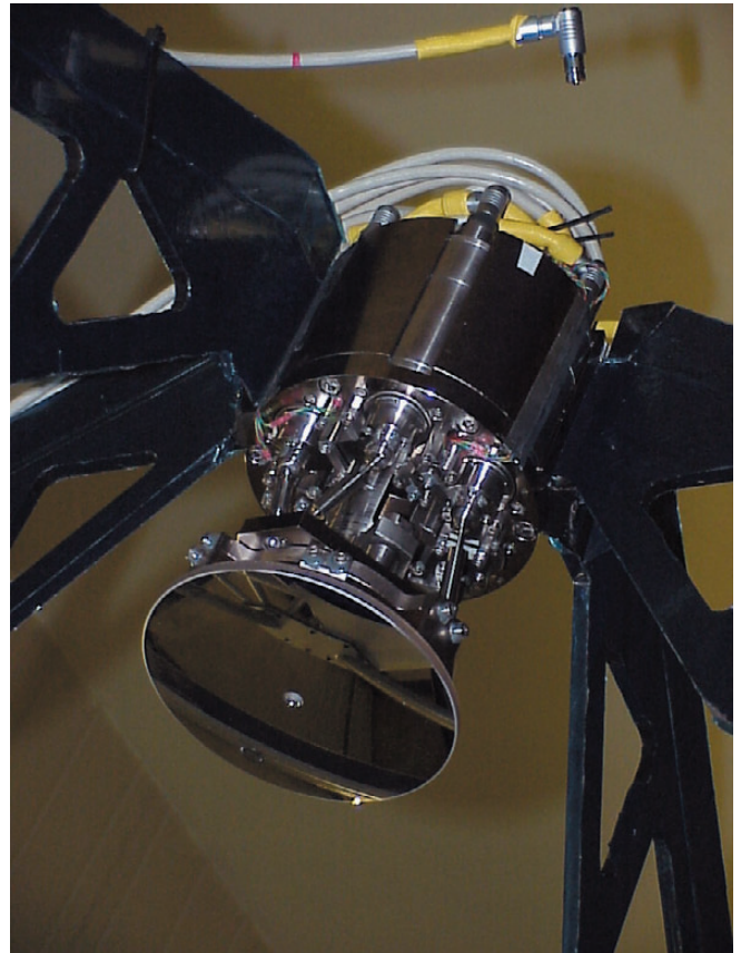
Figure 4: The 140-mm diameter secondary mirror is mounted on an hexapod to enable remotely controlled focus, centring and angular alignment. The hexapod, built by CSEM (Switzerland) is a very compact, very high accuracy mechanical device featuring a resolution smaller than 0.2 microns and a very small cross-coupling between focus and tilt motions to avoid mispointing while re-focusing the telescope. ▶
