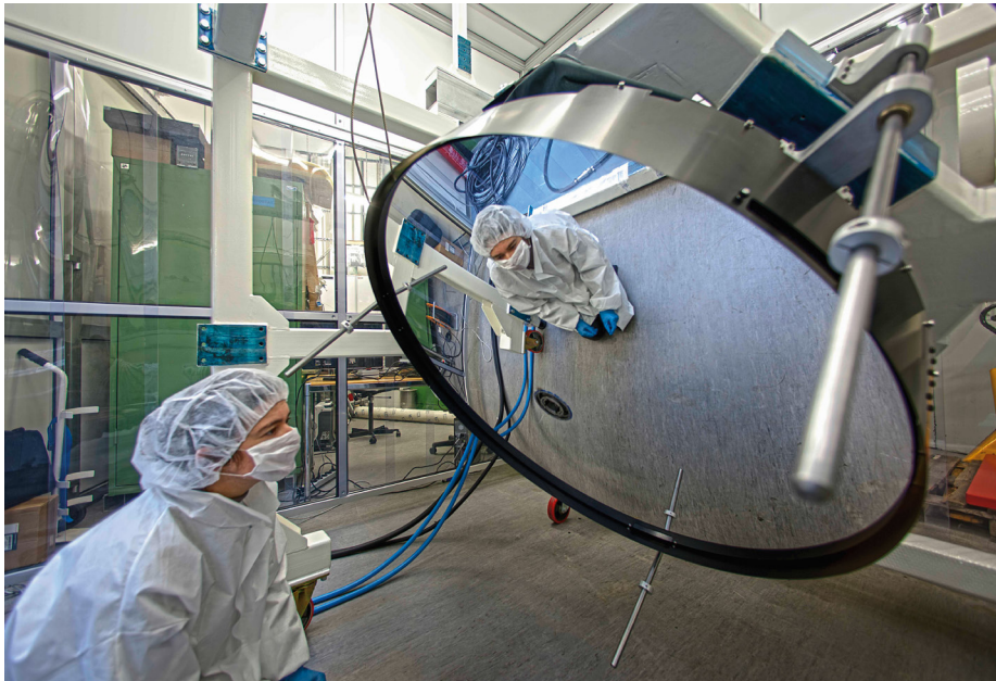
Figure 1. The deformable secondary mirror in its test stand. In operation the thin-shell mirror is held by the actuators with a gap of 65\ \mu\text{m} between the shell back face and the reference body front face. The black metallic structure surrounding the mirror is called the "EMC skirt" and shields the system from electromagnetic interference.
