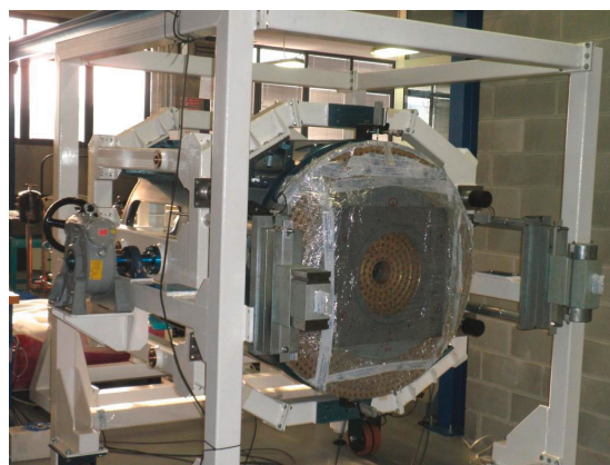
Figure 2. Finite element modelling of the complete DSM shown on the left. It is used as a baseline to compare with the experimental results. On the right, the hub with dummy weights and external encoders to measure flexure. The hub integration and service stand allows the inclination of the hub to be varied to characterise the flexure at the level of the reference body for different orientations. The results of the flexure campaign confirmed the system rigidity at 150\ \text{N/mm} .
