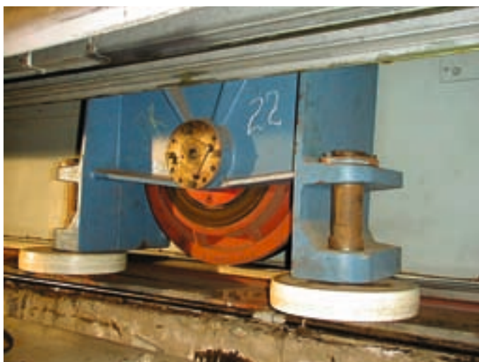
Figure 2: One of the original dome bogies, with the large centred wheel and rubber rim, is shown.
