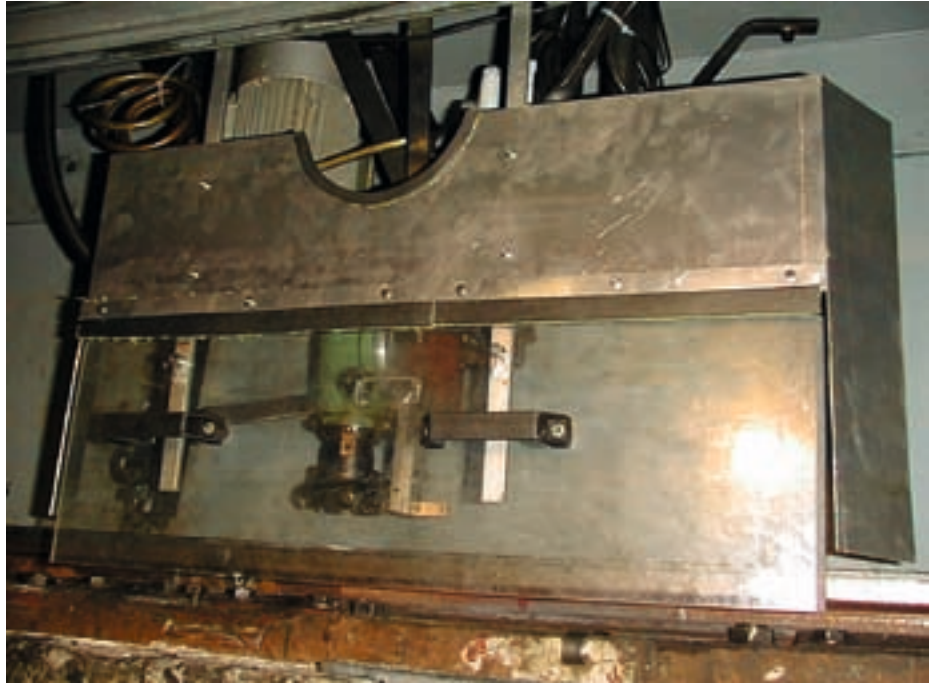
Figure 5: The special milling head, fabricated to machine the rail, attached to the dome.
