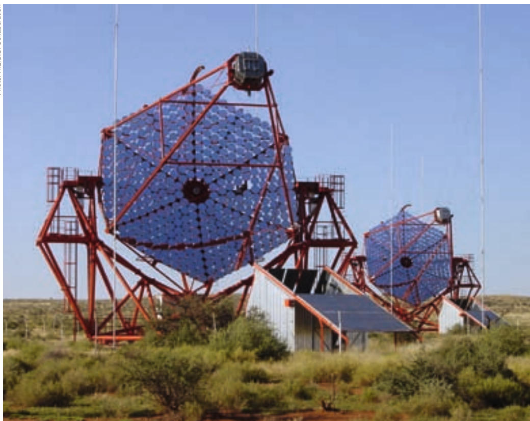
Two of the four H.E.S.S. Cherenkov telescopes for detection of very high energy gamma rays are shown. The H.E.S.S. observatory is situated in Namibia, southern Africa. Each telescope has a mirror diameter of 12 m with a camera consisting of 960 photomultipliers. The four telescopes are coupled and work in stereoscopic mode.
