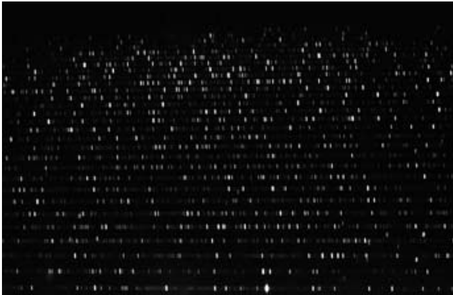
Figure 2: Spectrum of a thorium-argon calibration lamp with a 5 s exposure. 1500 lines are detected and 80 % are typically identified (calibrated) with the MIDAS/ECHELLE calibration procedure.
