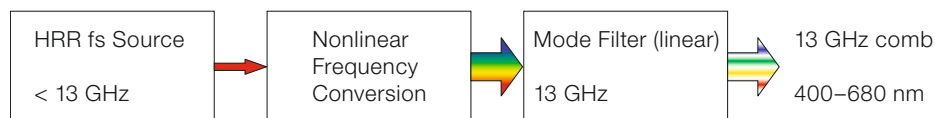
Figure 3 (above): Block diagram for the proposed laboratory demonstrator of the calibration system based on a frequency comb.
