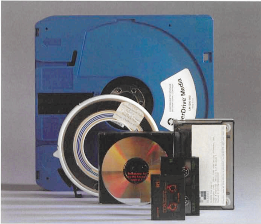
Figure 1: Optical disk; 9-track tape (for comparison); CD-ROM; QIC; Exabyte; DAT (front).
