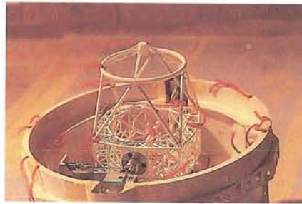
Figure 3: Flow visualization with wool tufts showing the recirculation pattern in the recess.
