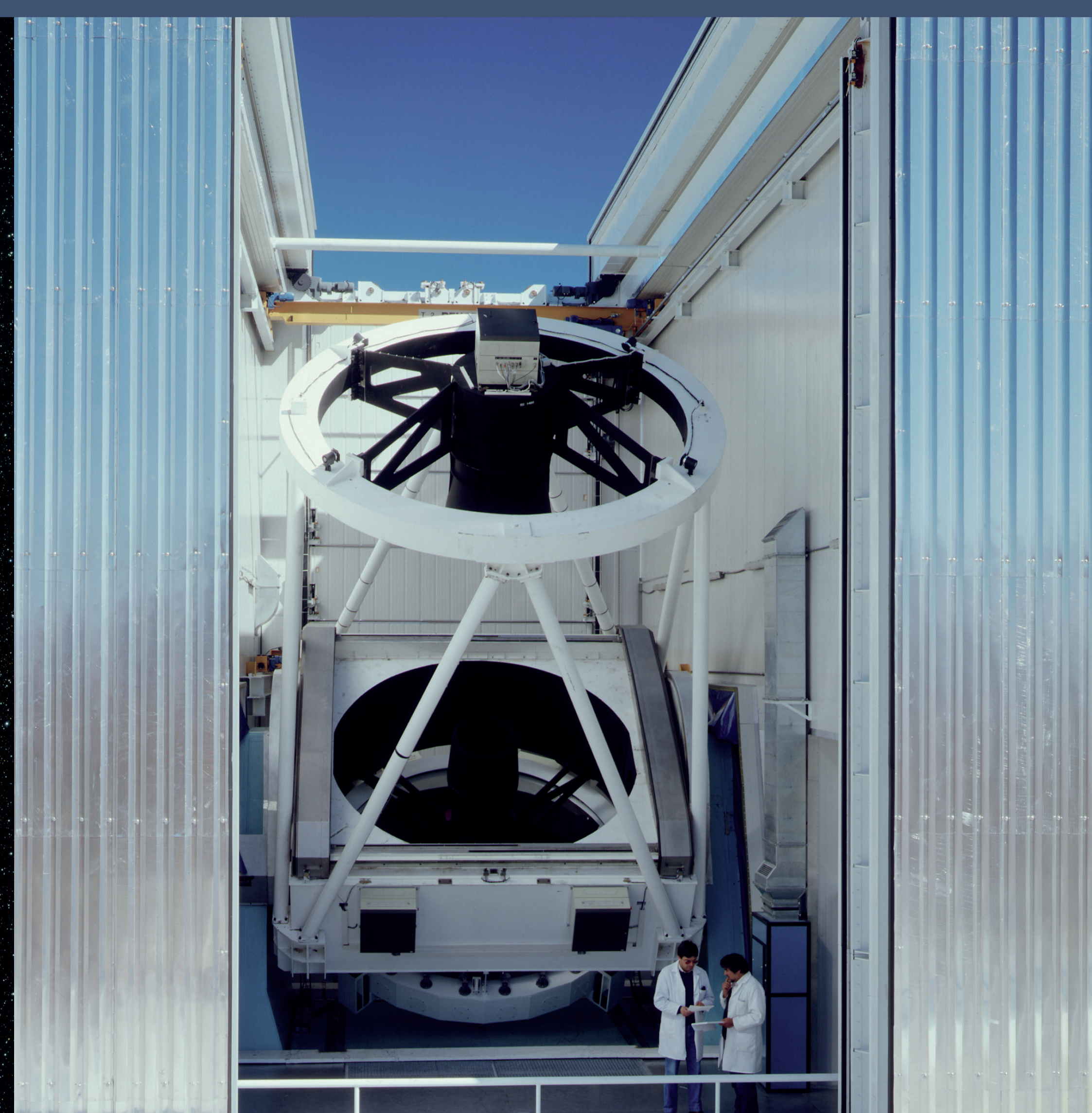
The revolutionary ESO 3.58-metre New Technology Telescope (NTT) in its octagonal enclosure. Credit: ESO/C. Madsen
