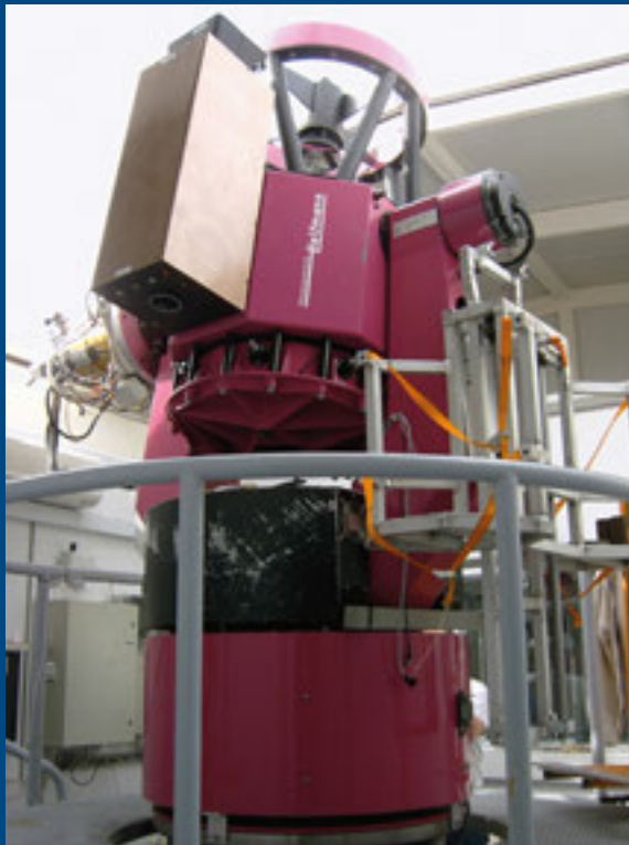
The Rapid Eye Mount telescope A 60-centimetre robotic telescope in a small dome, operated by Italian astronomers. The main purpose of the REM Telescope is to follow up promptly the afterglows of gamma-ray bursts.
