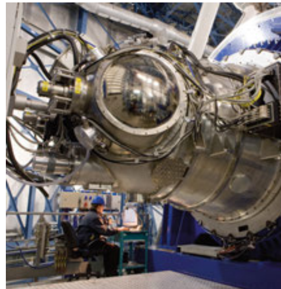
HAWK-I The HAWK-I instrument mounted on Yepun, Unit Telescope 4 of ESO's Very Large Telescope. HAWK-I covers about one tenth the area of the full Moon in a single exposure. It is uniquely suited to the discovery and study of faint objects, such as distant galaxies, young stars and planets.
