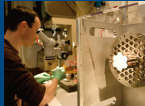
Active Phasing Experiment Components of the Active Phasing Experiment designed to validate technologies for accurate alignment of the segmented mirror of the forthcoming E-ELT.
