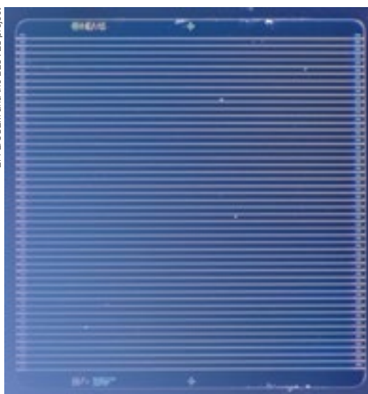
Close-up of a prototype photonic chip for an astrocomb. The waveguides are visible as horizontal lines. The chip is about 5 mm on each side.
