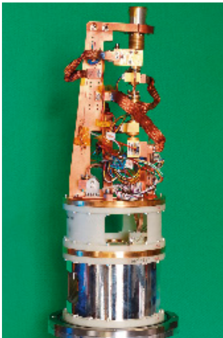
Fully assembled ALMA Band 2 prototype cold cartridge assembly in Bologna at the INAF iALMA/ Cryowaves laboratory.
