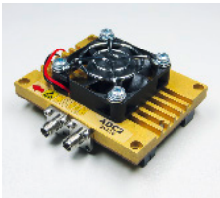
The Micram digitiser is being tested at the Université de Bordeaux. This digitiser can improve the overall system efficiency of ALMA and provide a significant increase in the instantaneous bandwidth.
