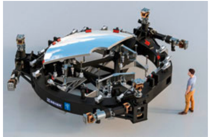
Preliminary design of the M2 cell developed by SENER.
