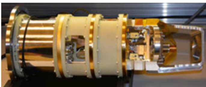
ALMA Band 5 receiver cold cartridge assembly at the OSF, ready for integration into an ALMA Front End.
