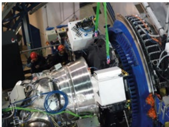
Installation of GRAAL on UT4. HAWK-I is the shiny metallic structure on the left while the blue part on the right is the Nasmyth A adapter/rotator. GRAAL is the black structure lying in between.
