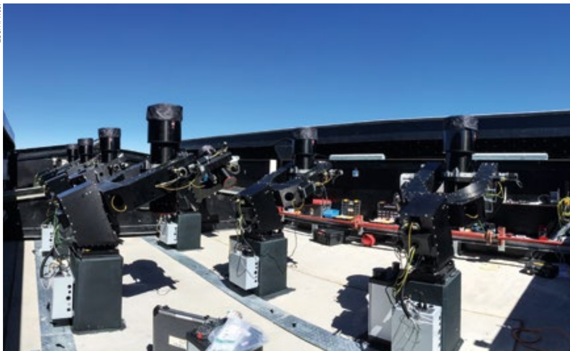
Part of the array of 20-centimetre telescopes of the hosted Next-Generation Transit Survey at Paranal.
