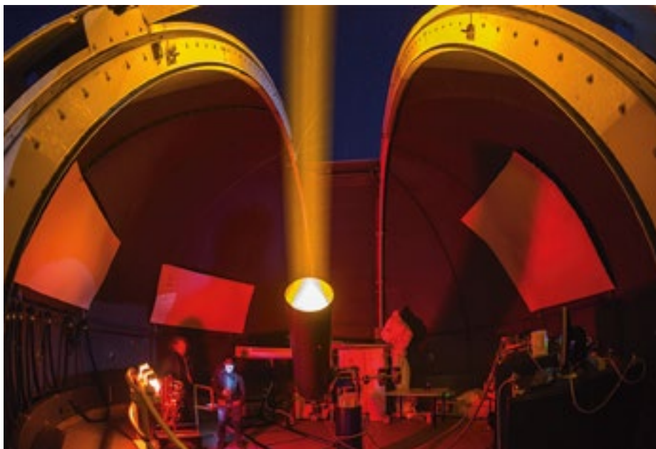
Laser Launch Telescope in the dedicated dome at the Observatorio de el Teide, propagating the laser beam during night-time observations.
