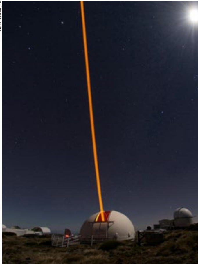
The transportable laser guide star system in operation on Mount Teide, Tenerife.
