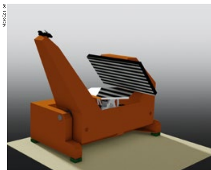
Conceptual design for measuring relative optical surface deformations of an E-ELT segment by deflectometry.
