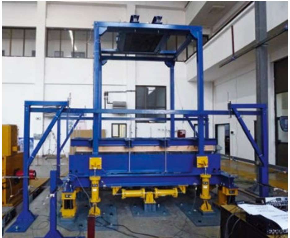
The seismic isolation test bed at ESO's Garching test facility. Both the lateral and the vertical components of the earthquake acceleration are significantly diminished through this isolation device, offering protection to both dome and telescope of the E-ELT.
