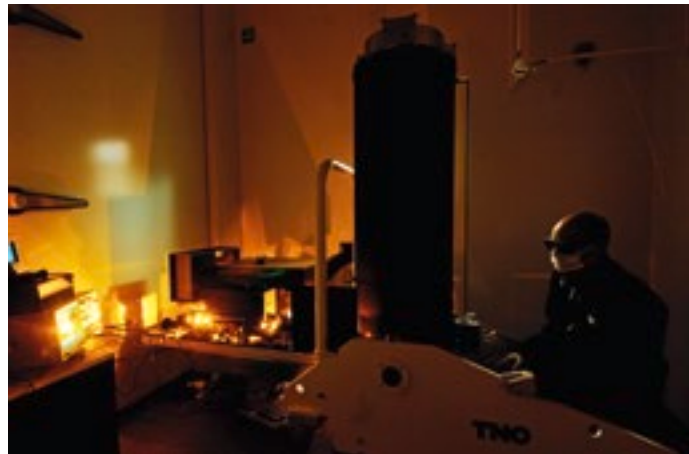
High-power laser test of the VLT's 4LGSF laser launch telescope in the ESO climatic chamber in Garching.
