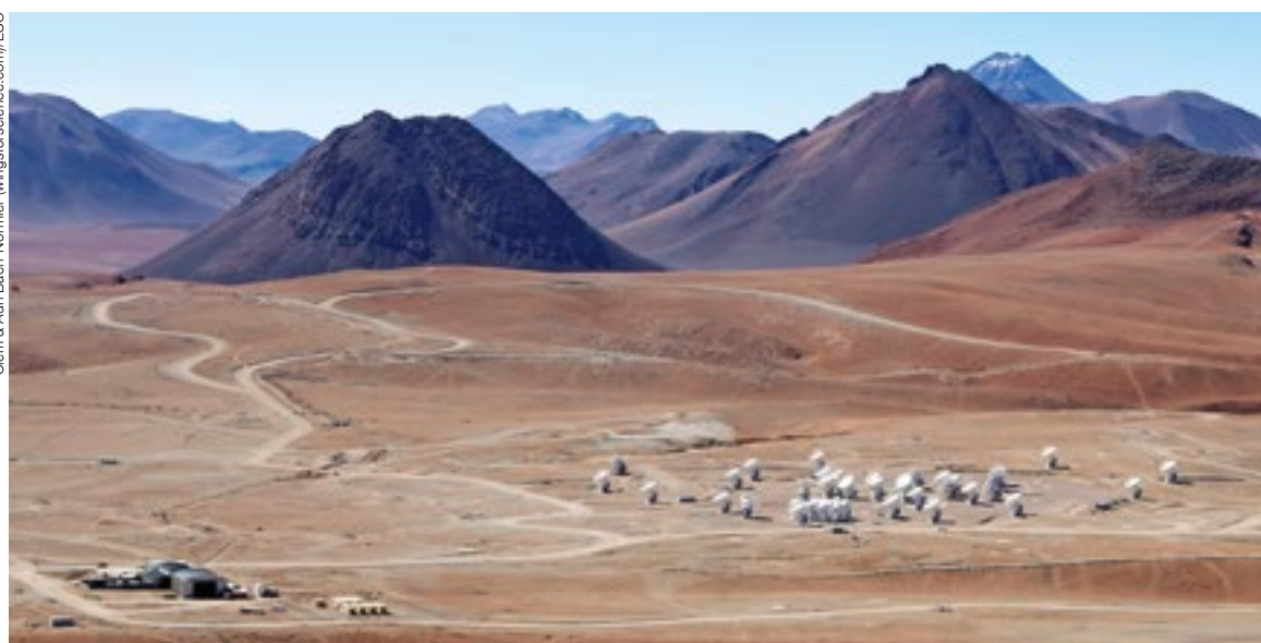
Aerial view of the Chajnantor Plateau, located at 5000 metres above sea level, where the array of ALMA antennas is located. The large antennas have a diameter of 12 metres, while 12 smaller antennas with a diameter of 7 metres make up the ALMA Compact Array.
