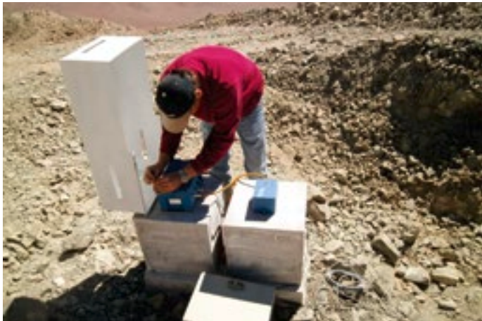
Installation of seismic station at Cerro Armazones.
