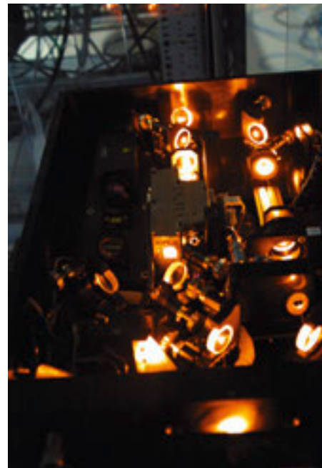
PARLA laser with its powerful yellow beam at the sodium wavelength of 589 nm.
