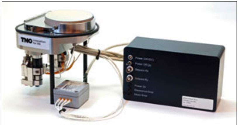
The 4LGSF optical test assembly on the test stand.
