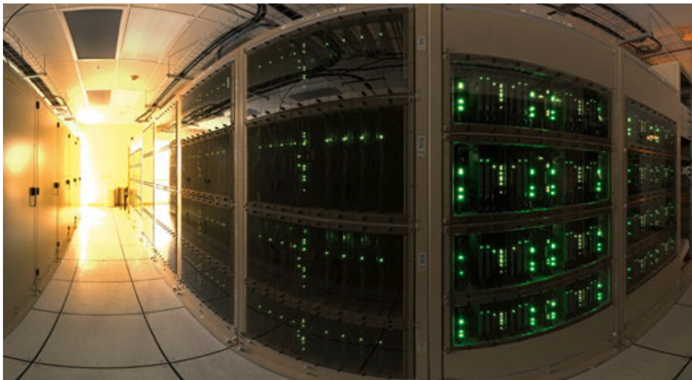
Wide-angle view of the racks in one of the four quadrants of the correlator at the AOS.
