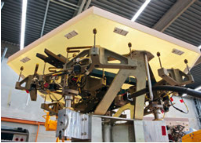
One segment of the giant primary mirror of the E-ELT undergoing testing at the Hochbrück warehouse in 2012.
