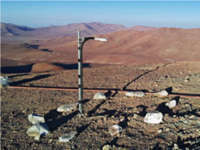
Net radiometer installed on the future E-ELT site.
