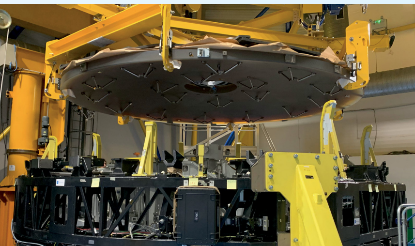
Removal of the M2 mirror from its cell at Safran Reosc.
