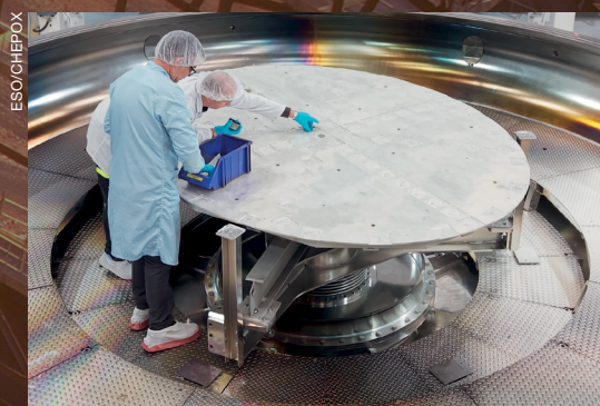
Inspecting mirror samples on the dummy M5 mirror during commissioning of the ELT's Large Coating Plant.
