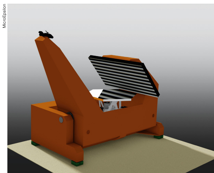
Conceptual design for measuring relative optical surface deformations of an E-ELT segment by deflectometry.
