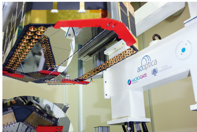
Adaptive mirror unit prototype for the E-ELT under test at AdOptica.
