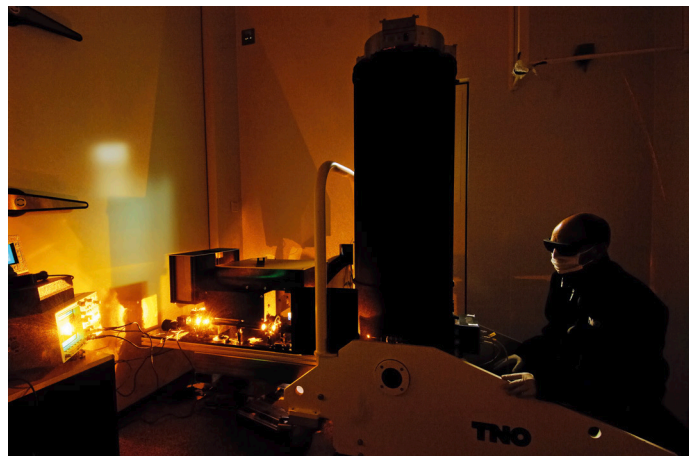
High-power laser test of the VLT's 4LGSF laser launch telescope in the ESO climatic chamber in Garching.
