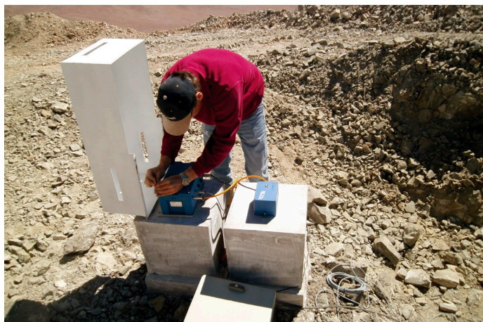
Installation of seismic station at Cerro Armazones.
