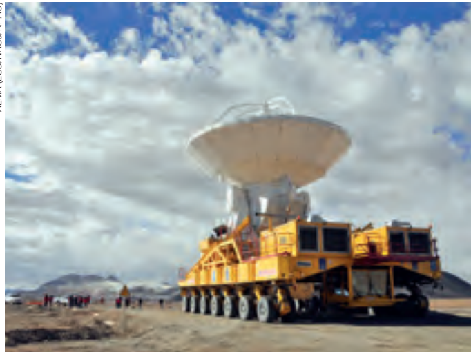
Transport of an ALMA antenna from the OSF (2900 m) to the AOS (5000 m).
