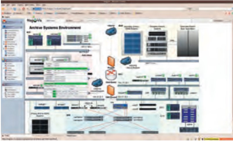
An example of the NAGIOS event monitoring system for the operational archive environment at ESO. This graphical overview provides real-time data, for instance for a Blu-ray production system.
