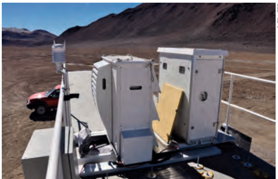
An ALMA external compressor enclosure (left) and internal electronic enclosure (right) undergoing environmental performance tests.
