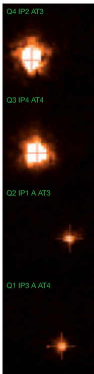
(Left) The four PRIMA beams (two stars per telescope) as seen in the VLTI laboratory on the infrared tip-tilt sensor IRIS.
