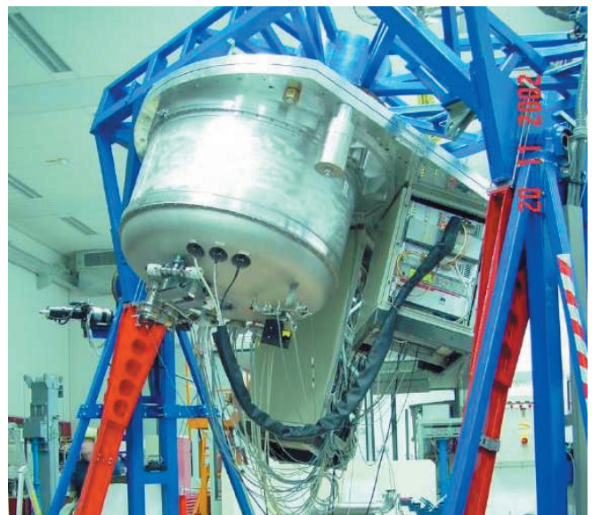
Left: end of October 2002 picture of the SINFONI adaptive optics module (top, blue) and the SPIFFI main structure (bare aluminium, below). Right: end of November 2002 picture of SPIFFI during flexure tests, as part of its Preliminary Acceptance in Europe.
