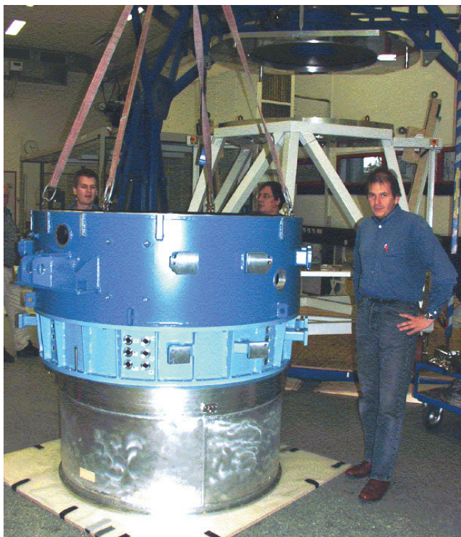
Left: end of October 2002 picture of the SINFONI adaptive optics module (top, blue) and the SPIFFI main structure (bare aluminium, below). Right: end of November 2002 picture of SPIFFI during flexure tests, as part of its Preliminary Acceptance in Europe.
