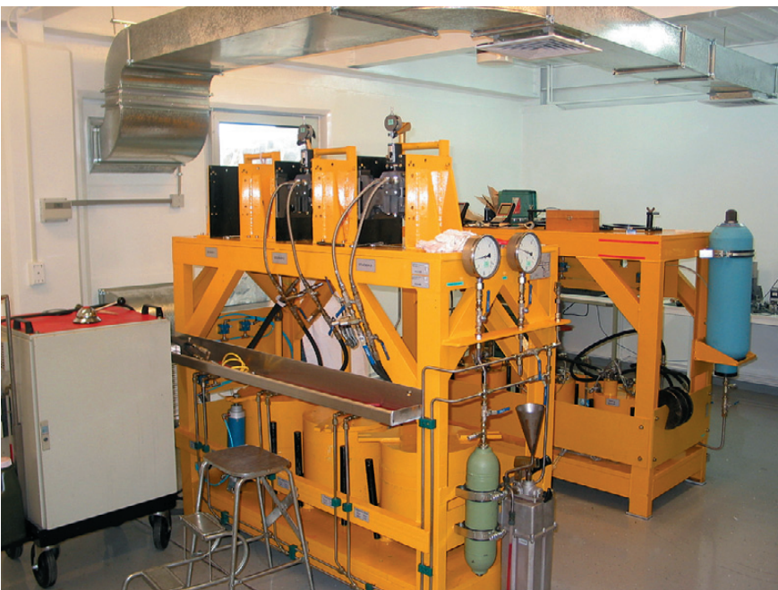
Test equipment in the new lab for the maintenance of VLT hydraulic supports.
