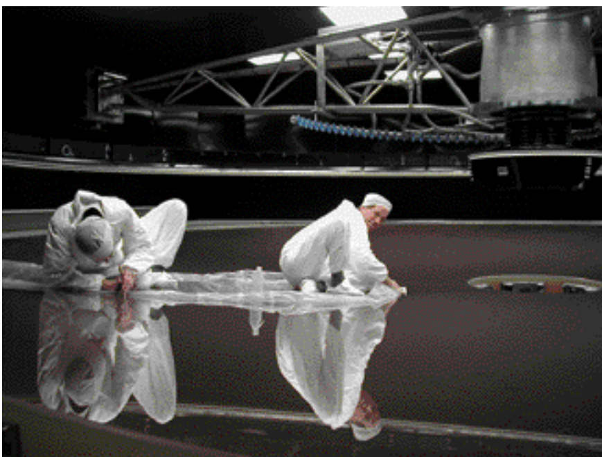
Figure 22: After removal of the third 8.2-m Zerodur mirror from its transport box, the protective layer is carefully removed before coating.
