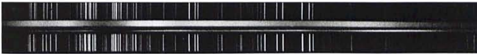
Two spectrograms of the 1972 supernova in NGC 5253 taken in Cassegrain focus with the 1.5 m telescope. The upper spectrogram is from May 17, 1972, the night after the announcement. The lower spectrogram is from August 28, 1972. The displacement of the very wide emission bands is obvious. In the upper spectrogram a sharp absorption line is faintly visible, originating from light absorption in interstellar calcium in our Galaxy.
