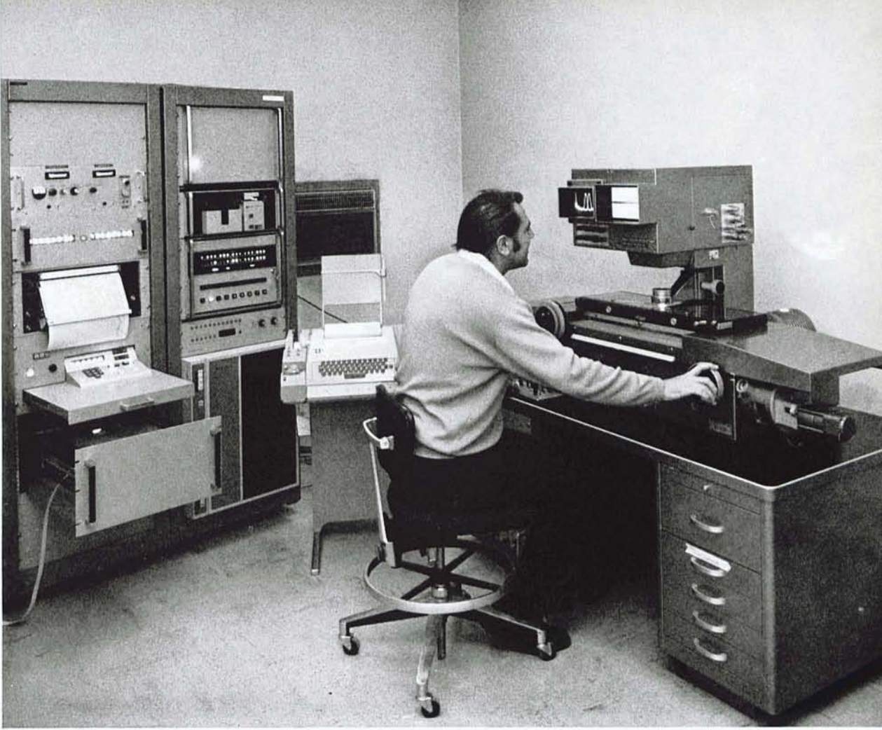
Automated Grant comparator-microdensitometer in the Vitacura Headquarters, Santiago. The data acquisition and control system is based on a HP 2114 B computer.
